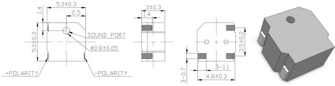
**Packaging:** Parts are supplied on tape-and-reel, 1000 pcs/reel. Units do not come with wash label and are not appropriate for aqueous wash.
